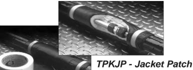
The jacket patch kits are used to seal a splice in a bundle or to extend the insulation and weatherproof jacket should the bundle be cut back too far during installation. They are used as a repair patch for any incidental field damage to bundles. The jacket patch kit is required with the optional line temperature sensing thermostat. Each kit contains thermal insulation, fiberglass tape and a self-sealing patch.
