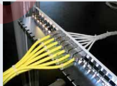
Alien Crosstalk arrangement by using MegaLineNet®: 6 "disturber" and 1 "victim"
