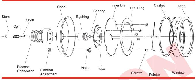
**Warning:** When selecting all bimetal thermometers, consider the media and the ambient operating conditions. Improper application can be detrimental to the thermometer and can cause failure and possibly personal injury or property damage. Inaccuracies resulting from improper setting of the external adjustment by the user may cause personal injury or property damage. Consult ASME B40.3 for guidance in selection and use of bimetal thermometers.
